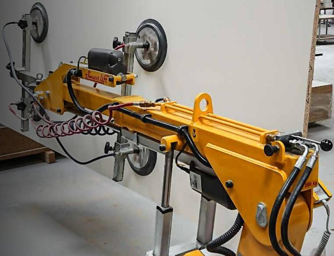
Dansk Boligstål in Aalborg makes special solutions for kitchens, work stations, and elevators, among other things. In the large halls, a pair of electric vacuum lifts help transport heavy items to and from the machines for processing.
